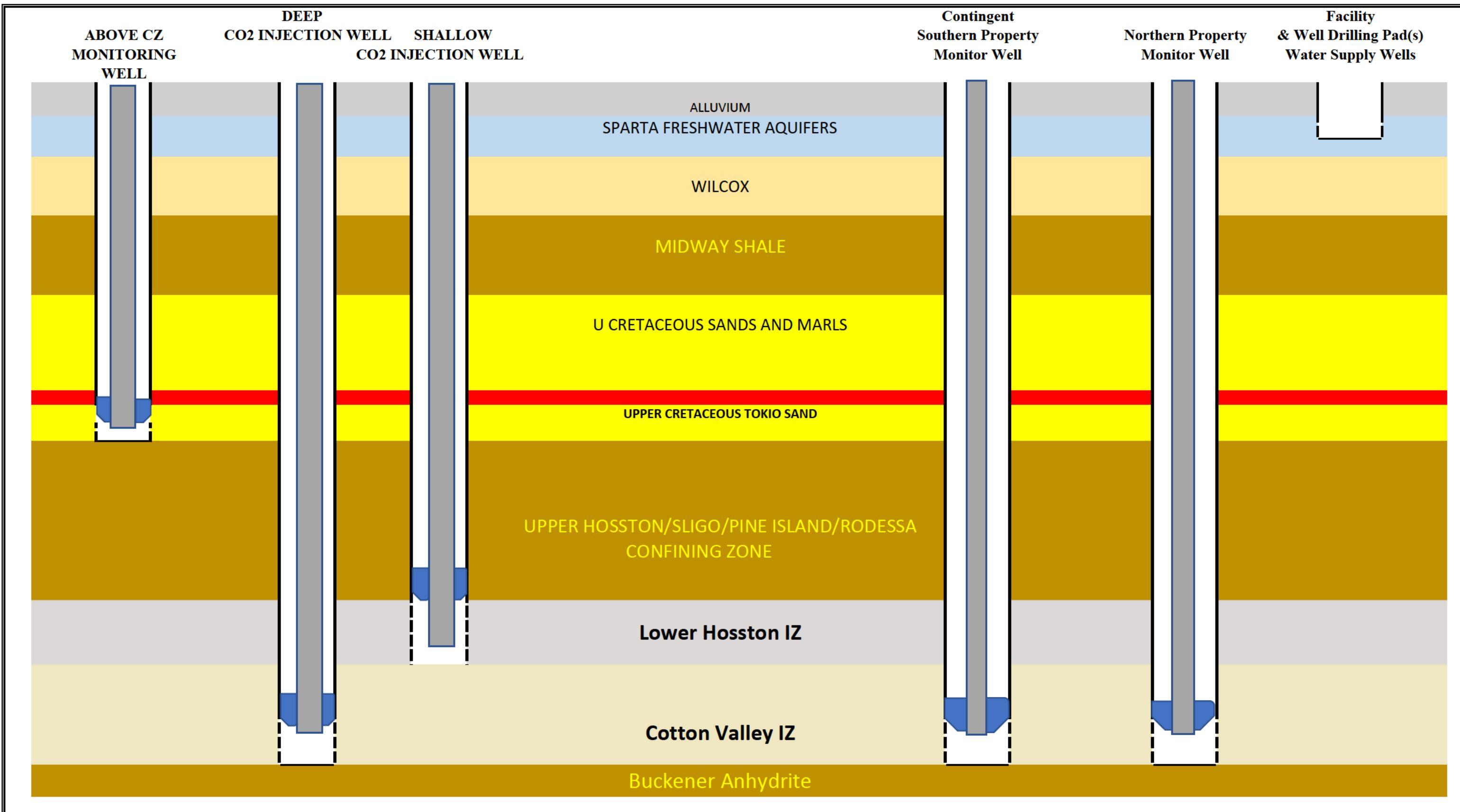
Figure 1 - Proposed Lapis Energy El Dorado Chemical Company Monitoring Schematic Illustration
