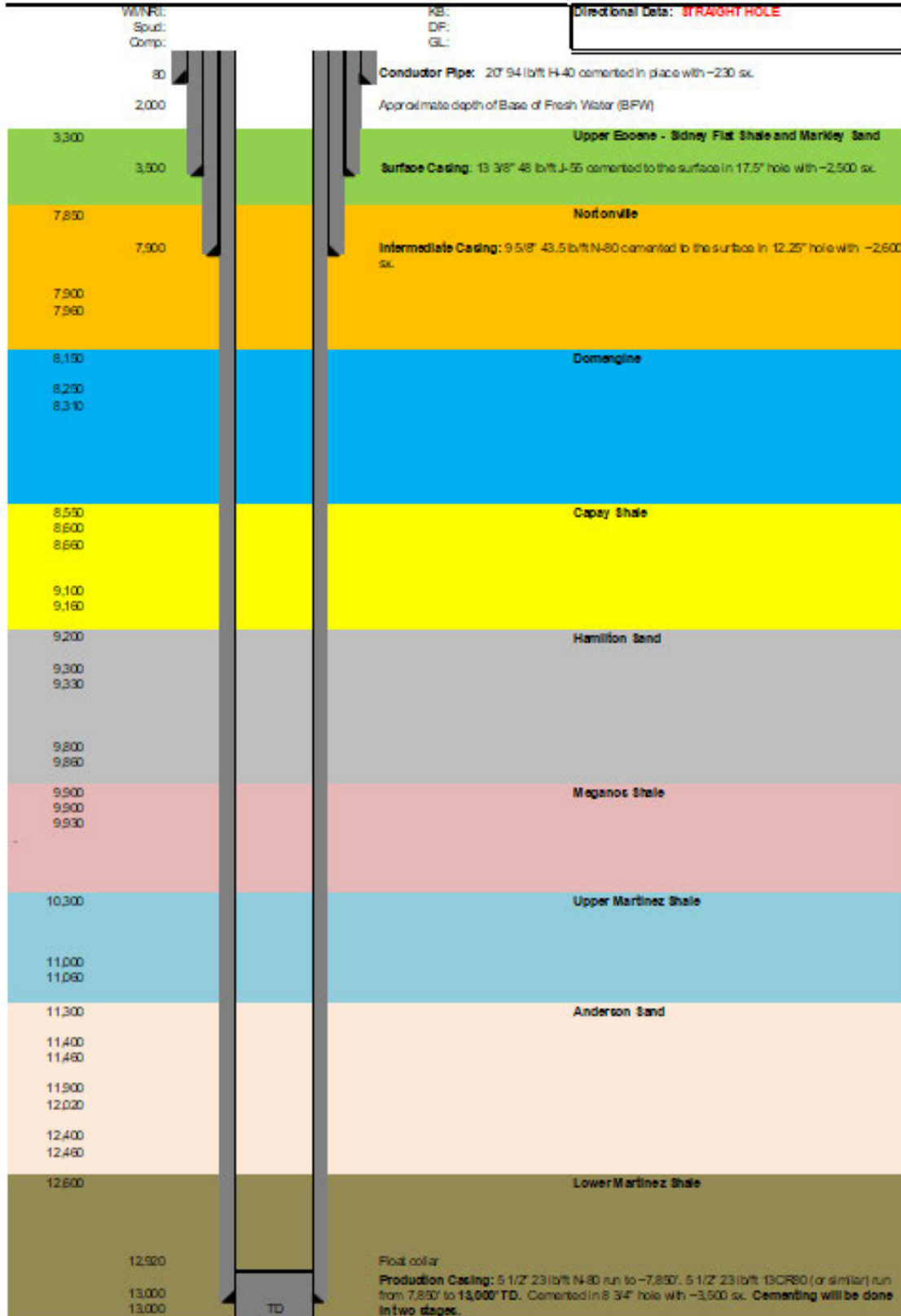
FIGURE A.II-1. SCHEMATIC OF IW-A1 IN INJECTION WELL SERVICE
