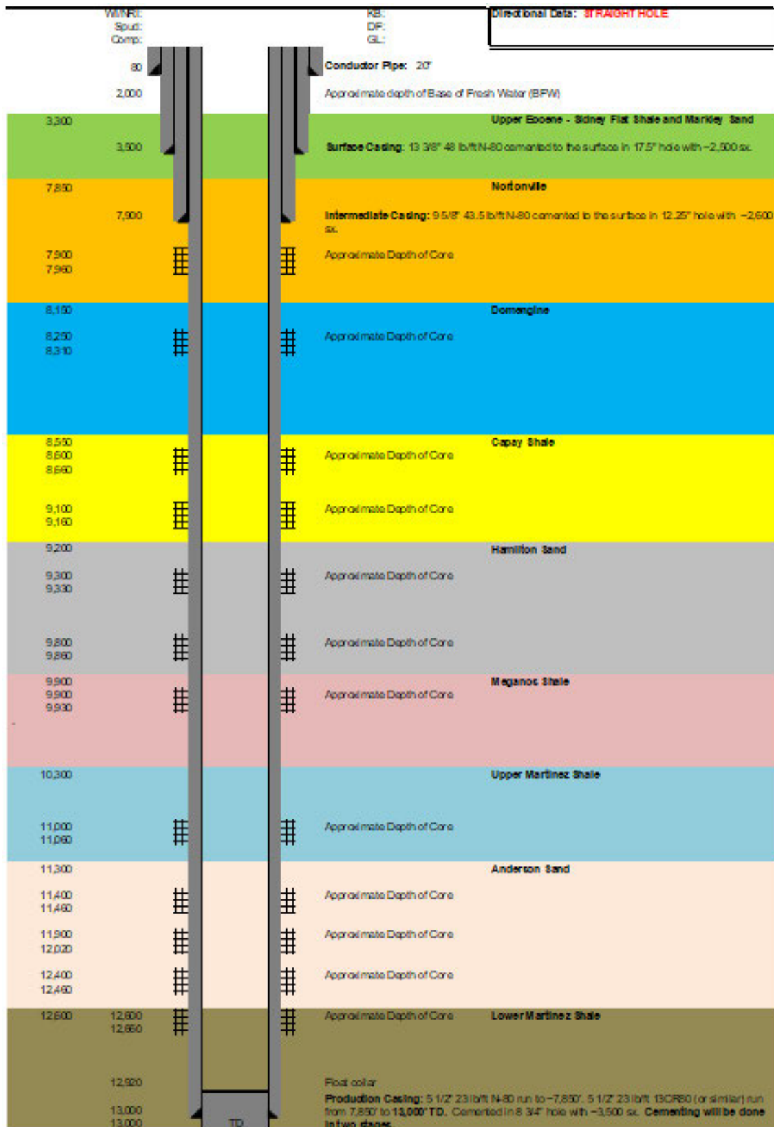
FIGURE A.II-3. DRAFT SCHEMATIC OF IZMW-A1
