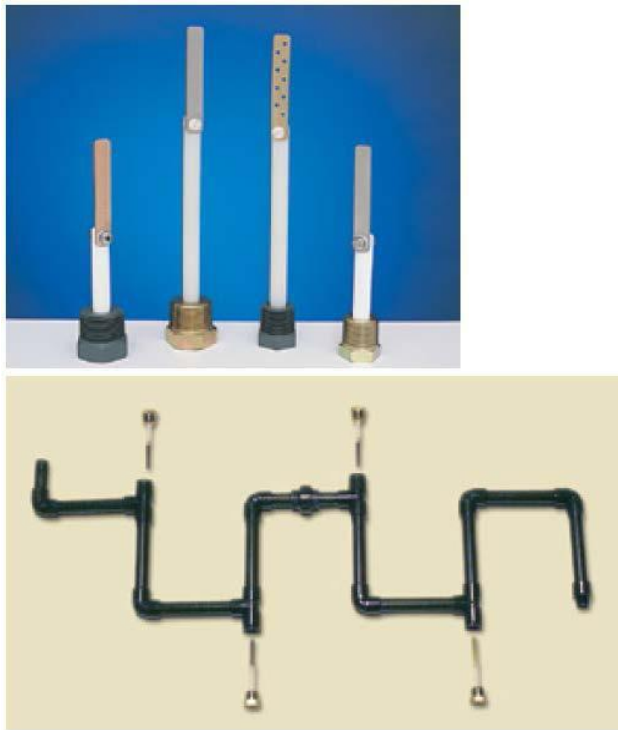
Figure 3. Coupon holder (top). Flow-through pipe arrangement (bottom).
