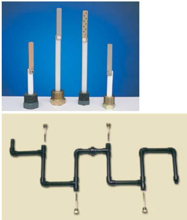
Figure 3. Coupon holder (top). Flow-through pipe arrangement (bottom).
