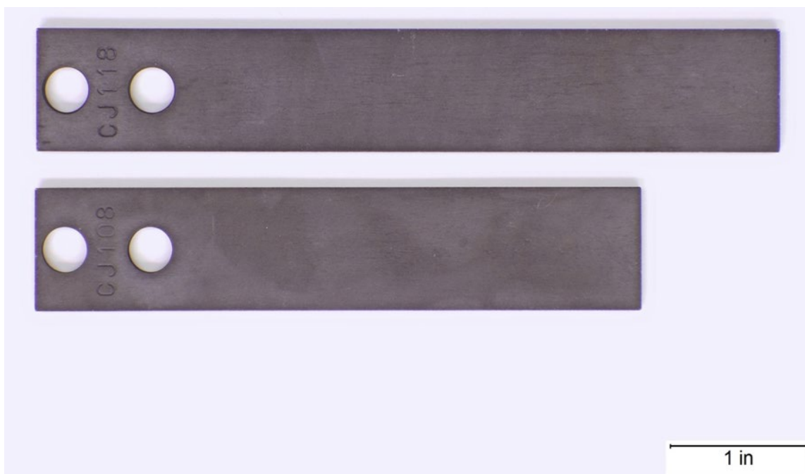
Figure 7: Type of corrosion coupons to be used for corrosion monitoring (Cosasco, 2022).
