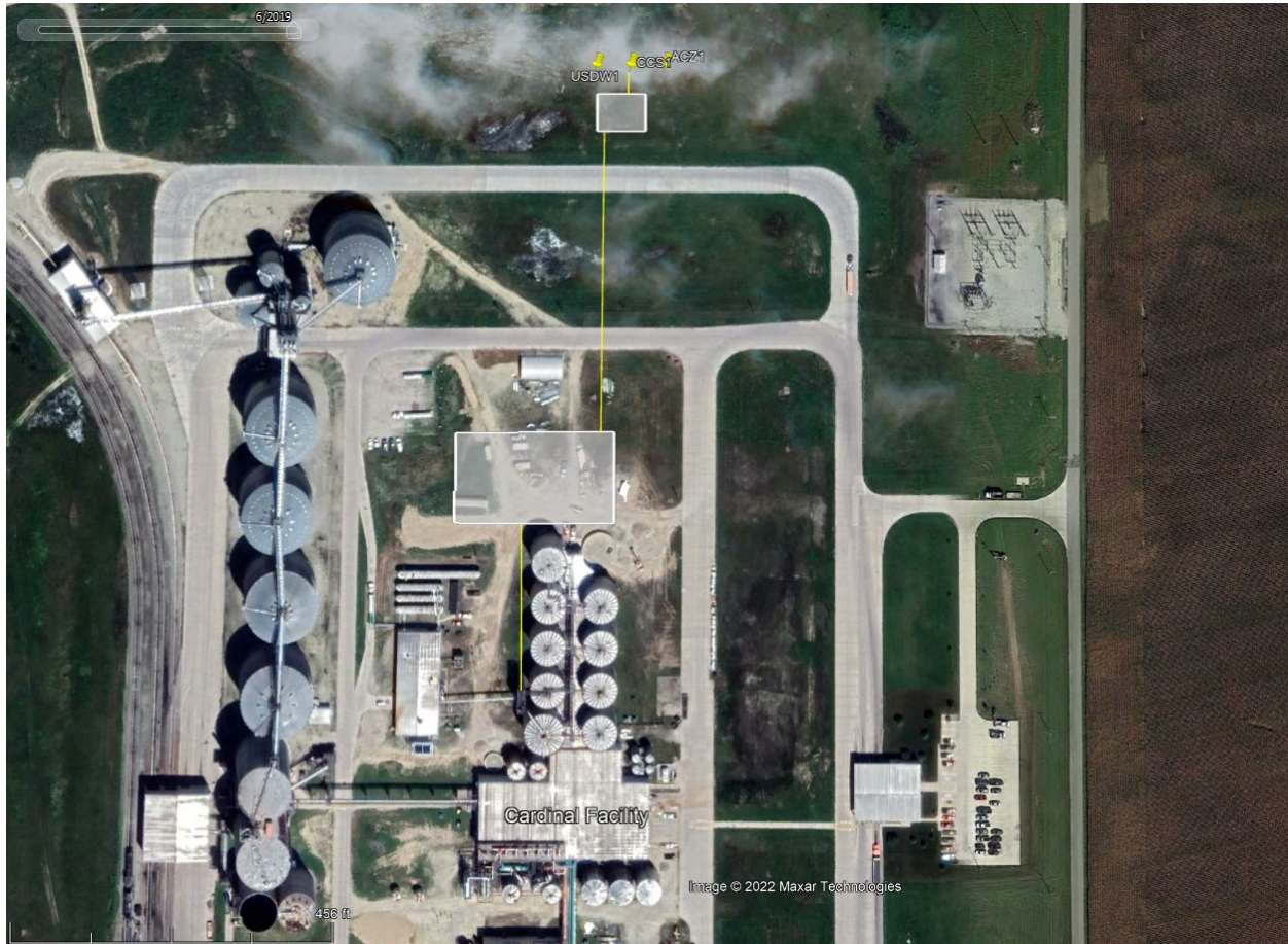
Figure 3. Ethanol Facility, flowlines, surface capture facility, CCS1, proposed lowermost USDW monitor well (USDW1), and proposed above confining zone monitoring well (ACZ1) location.
