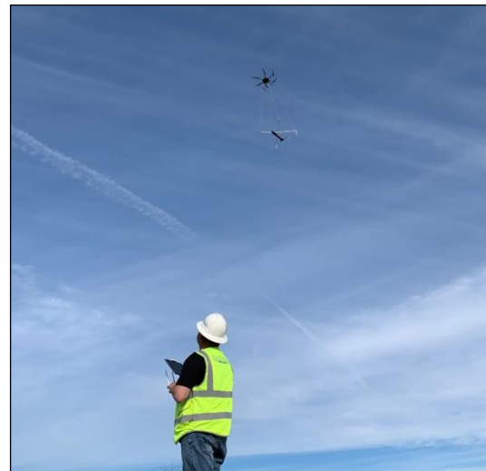
Figure 2: PIC navigating UAV and magnetometer payload to begin surveying.
