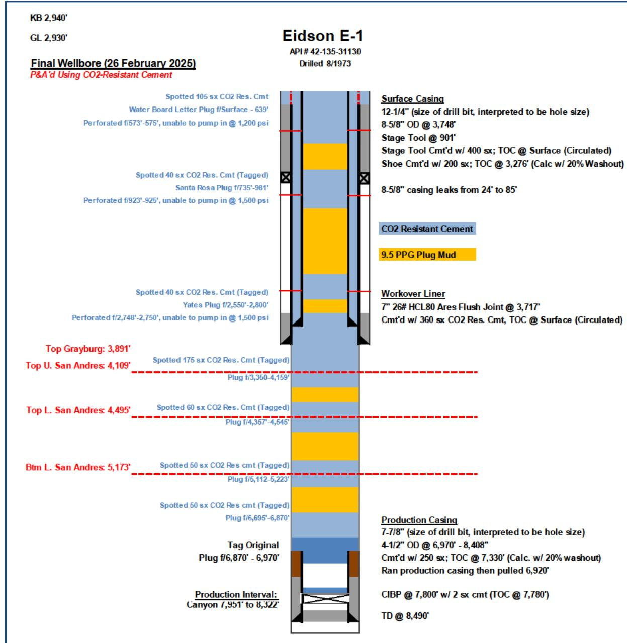
Figure 99. Wellbore diagram following corrective action on Eidson E-1 (4213531130).
