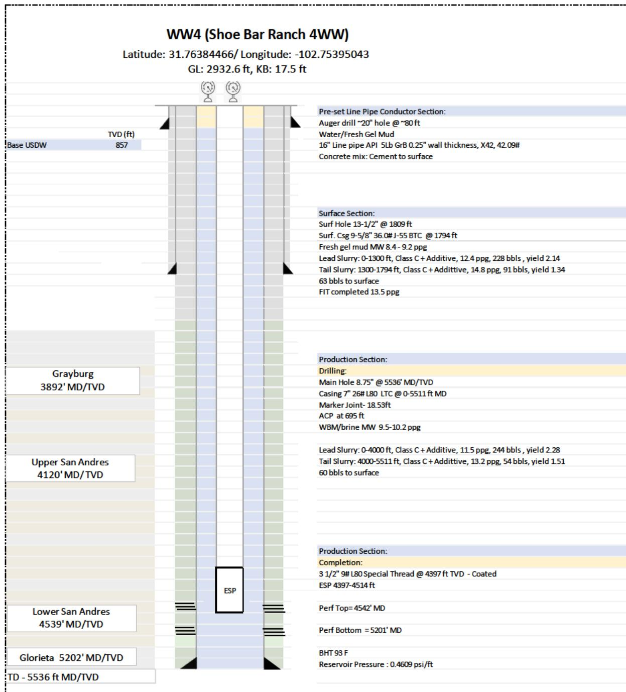
Figure 9. As-built wellbore diagram for WW4.
