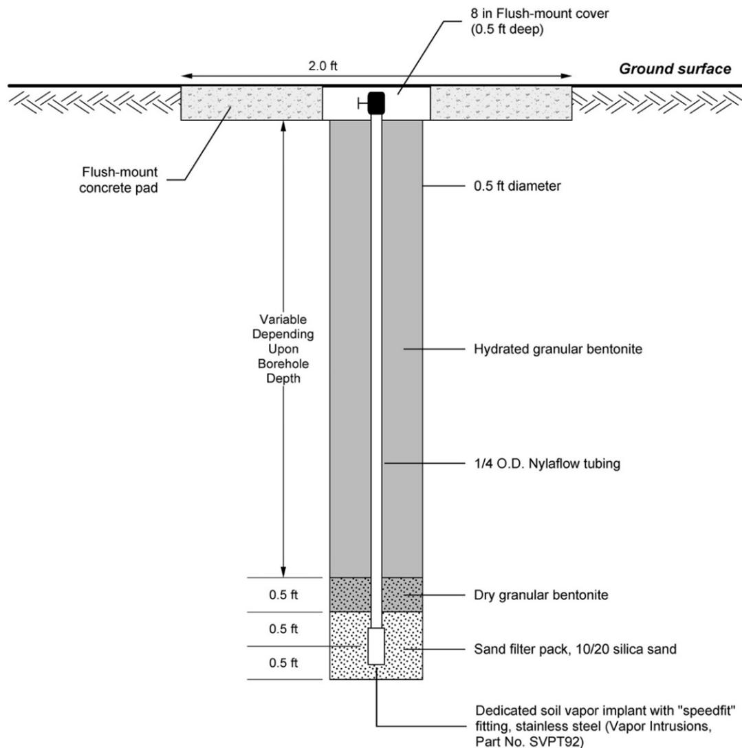
**Figure 65. General soil gas probe station construction schematic for BRP Project.**
