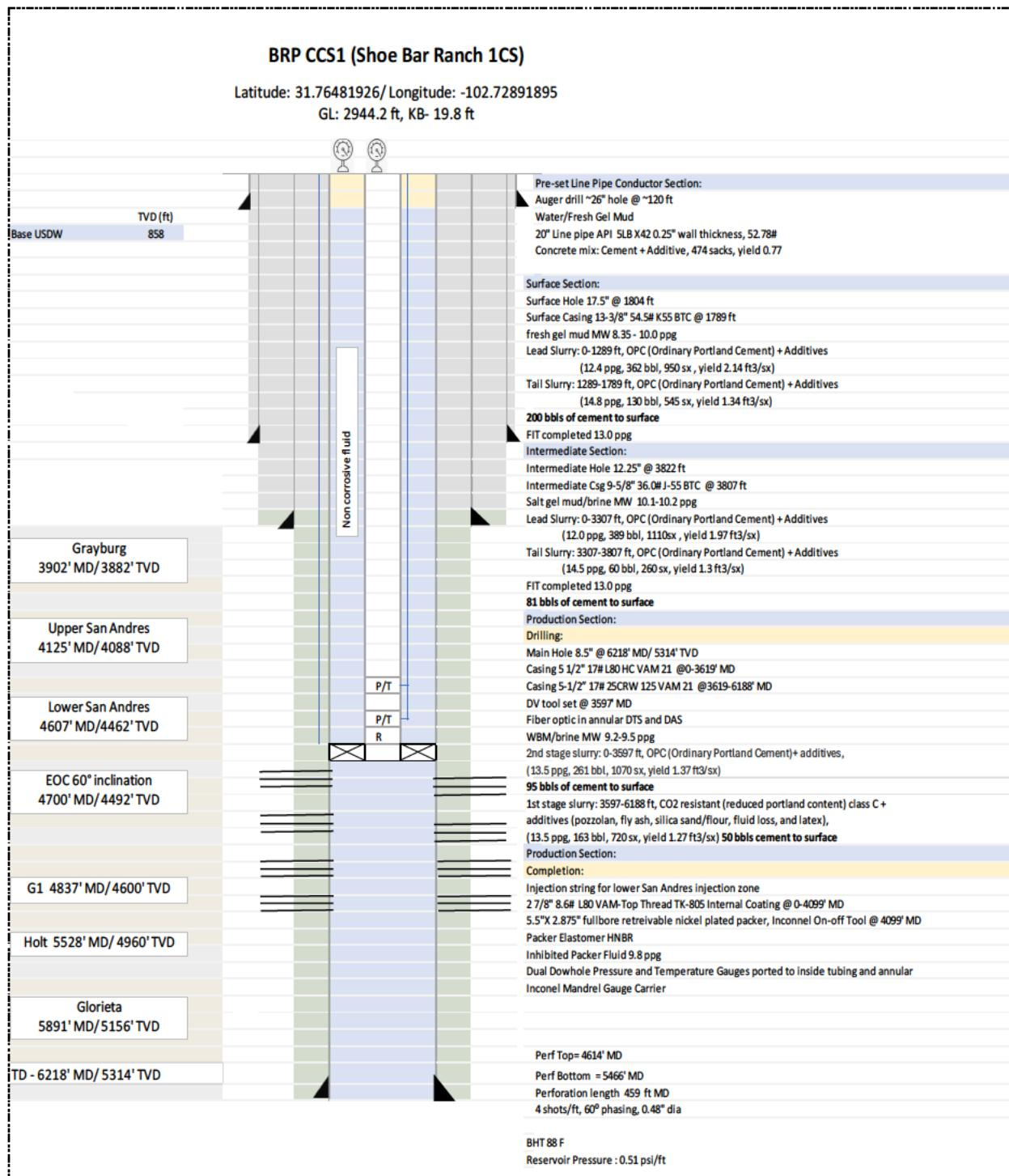
Figure 1. As-built wellbore diagram for BRP CCS1.
