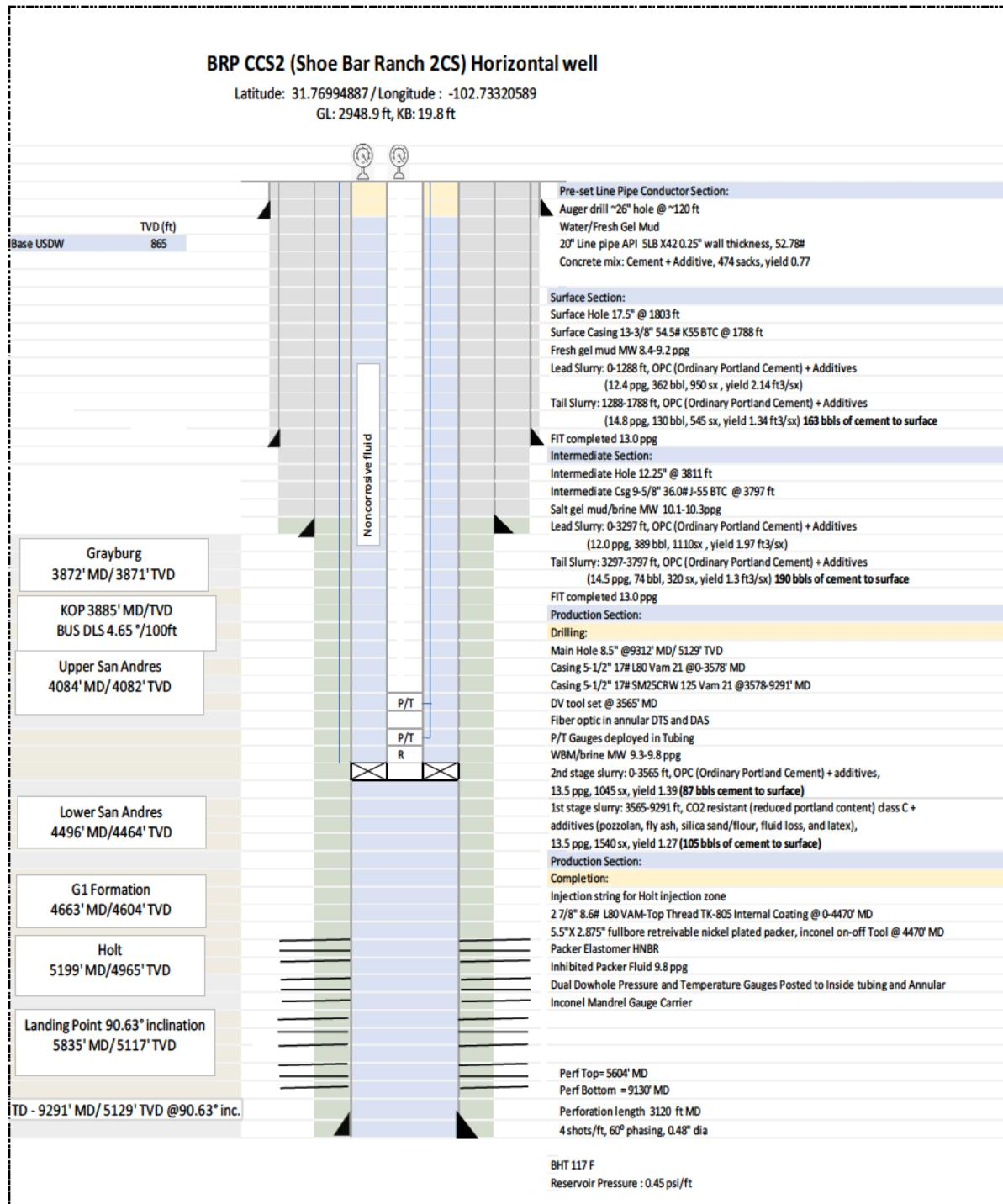
Figure 2. As-built wellbore diagram for BRP CCS2.
