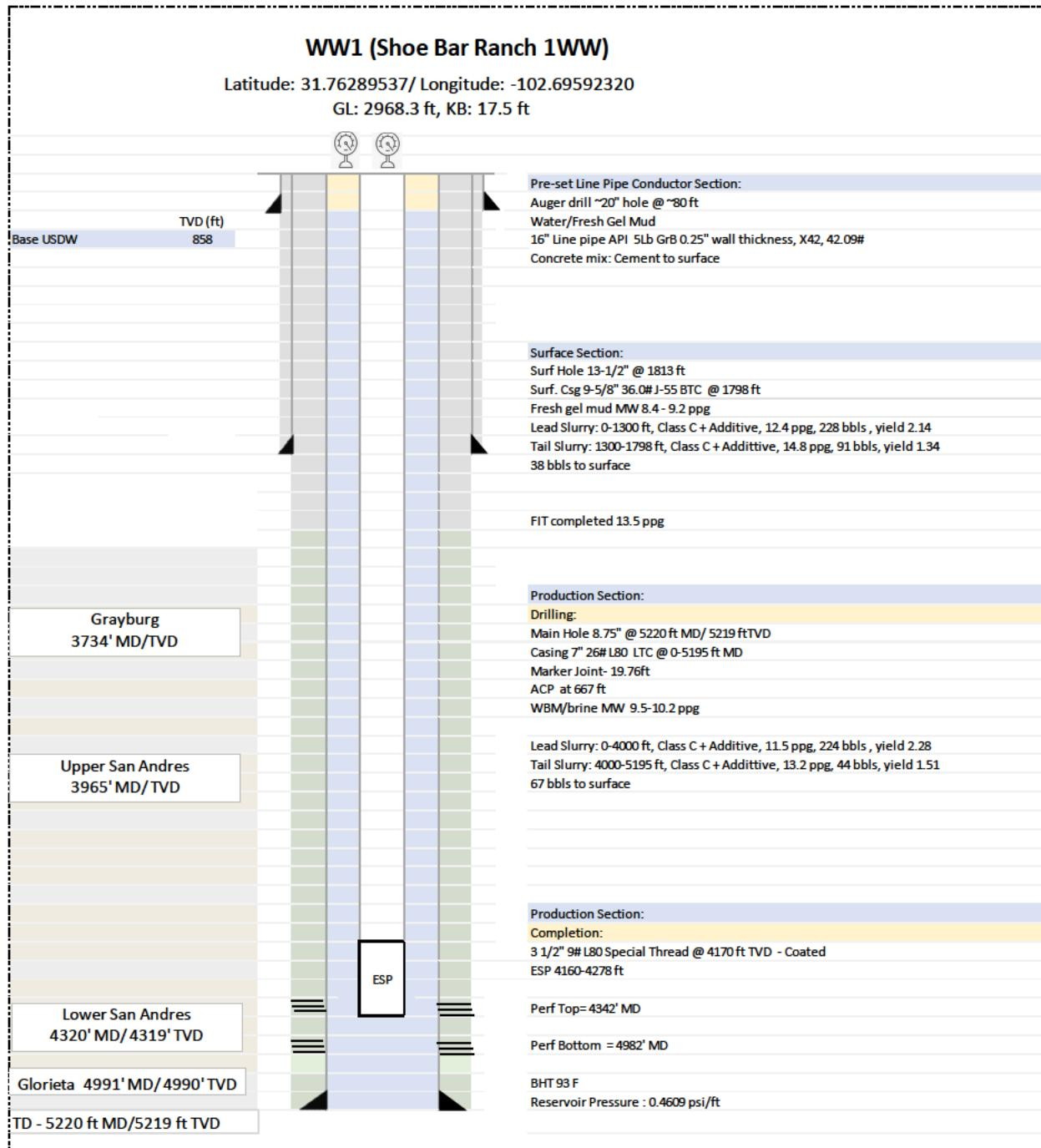
**Figure 6. As-built wellbore diagram for WW1.**
