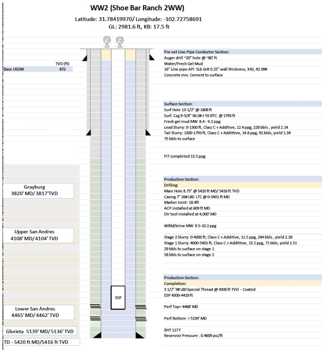
**Figure 7. As-built wellbore diagram for WW2.**
