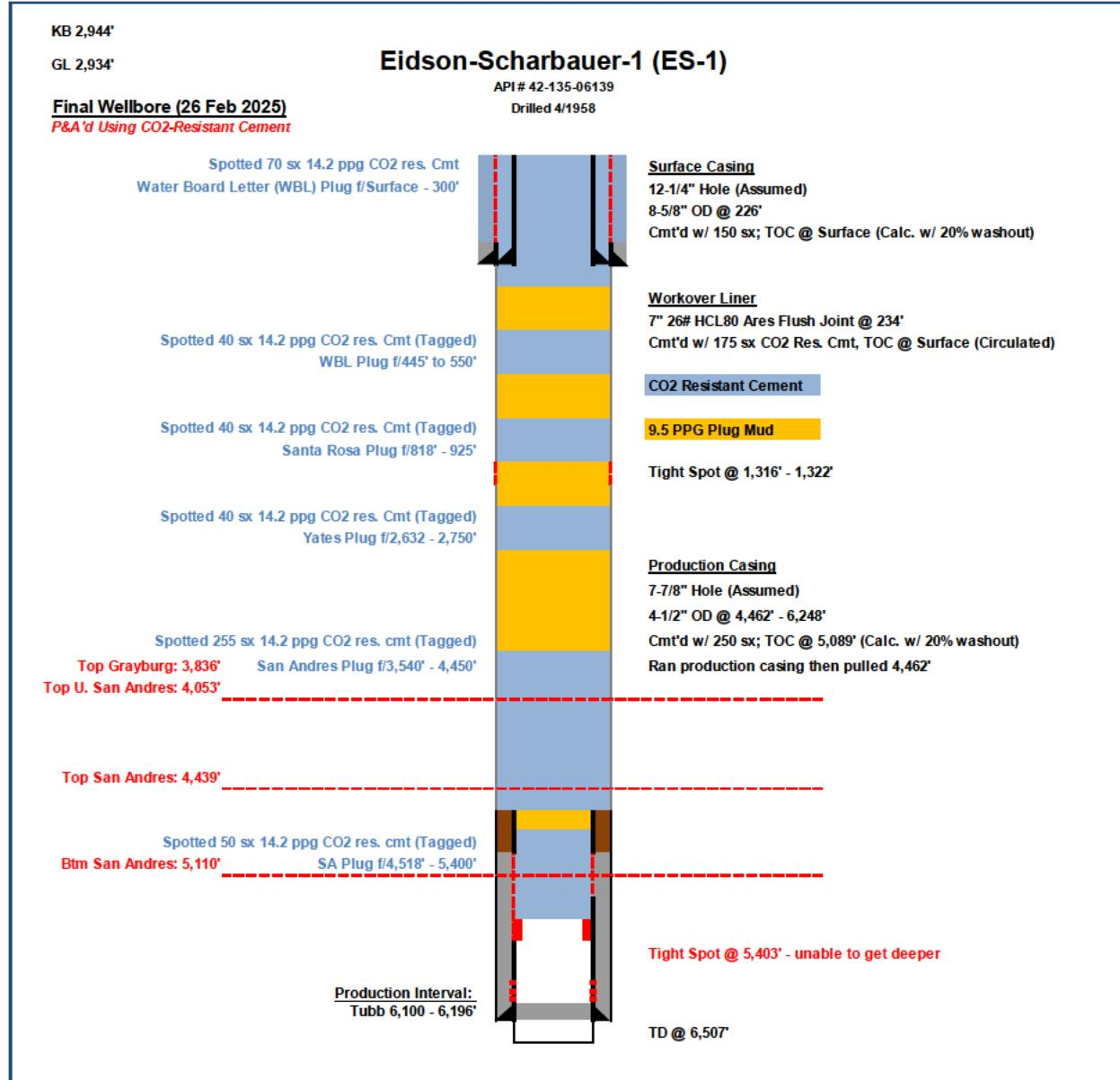
Figure 97. Wellbore diagram following corrective action for Eidson-Scharbauer-1 (4213506139).
