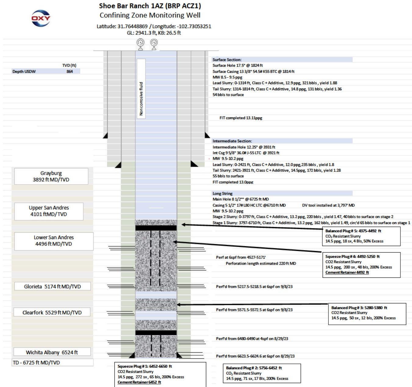
**Figure 11. As-built wellbore diagram for ACZ1.**
