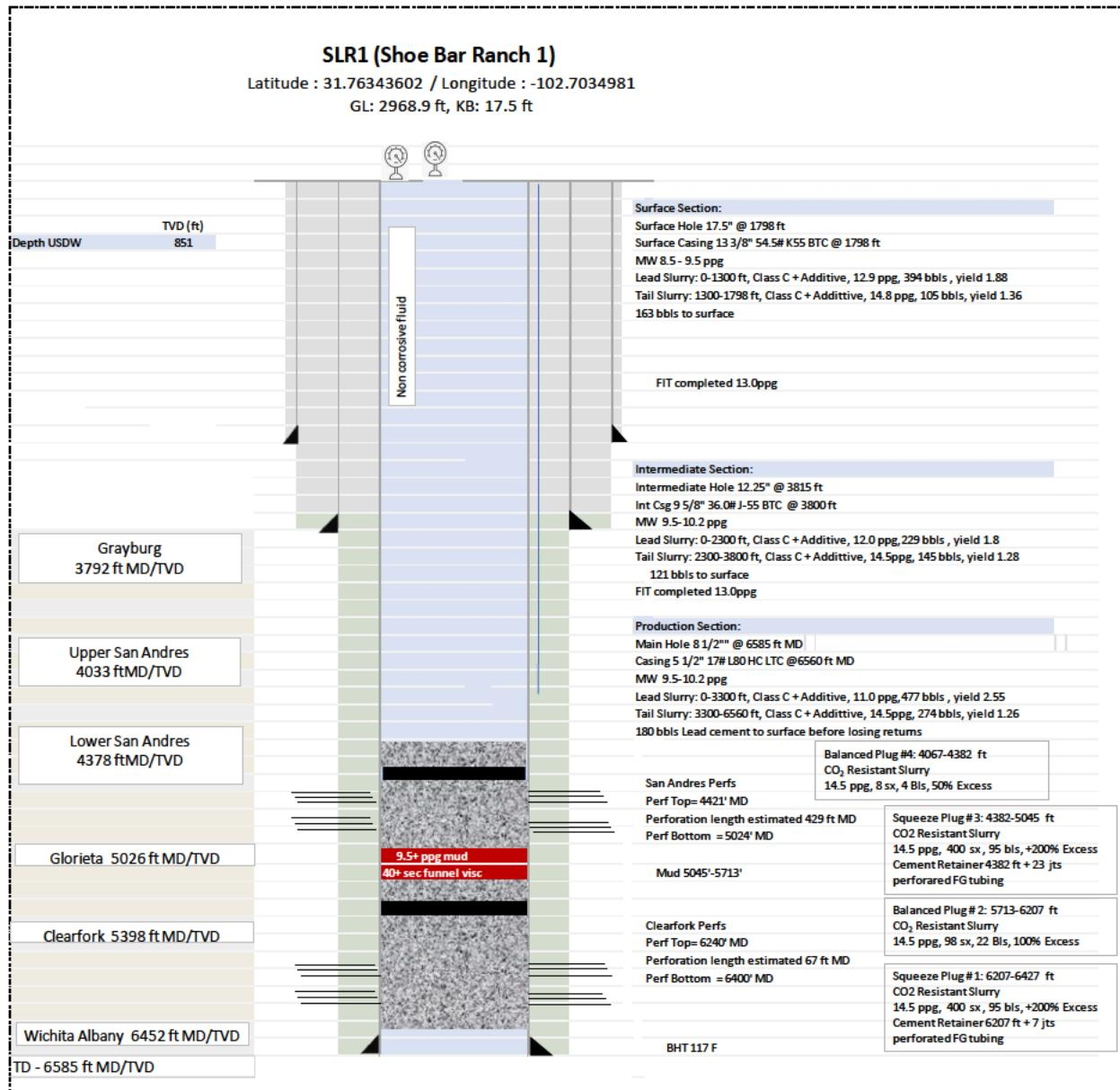
**Figure 10. As-built wellbore diagram for SLR1.**
