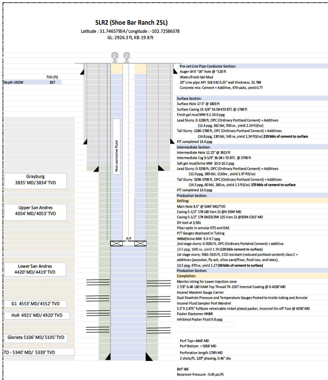
**Figure 4. As-built wellbore diagram for SLR2.**
