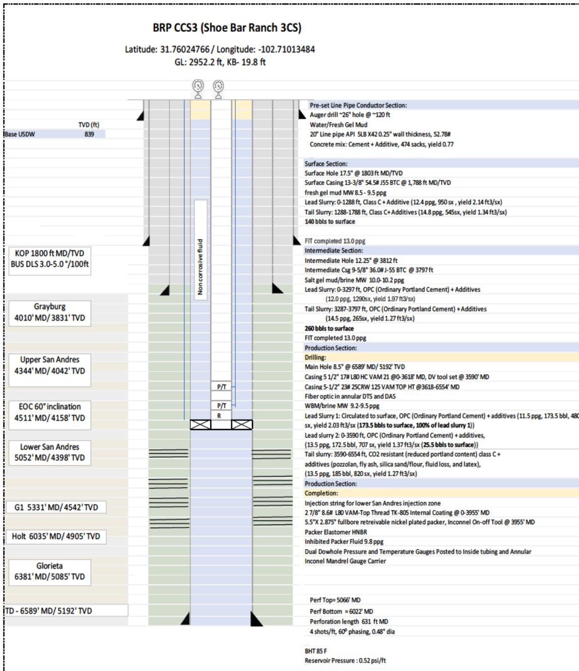
Figure 3. As-built wellbore diagram for BRP CCS3.
