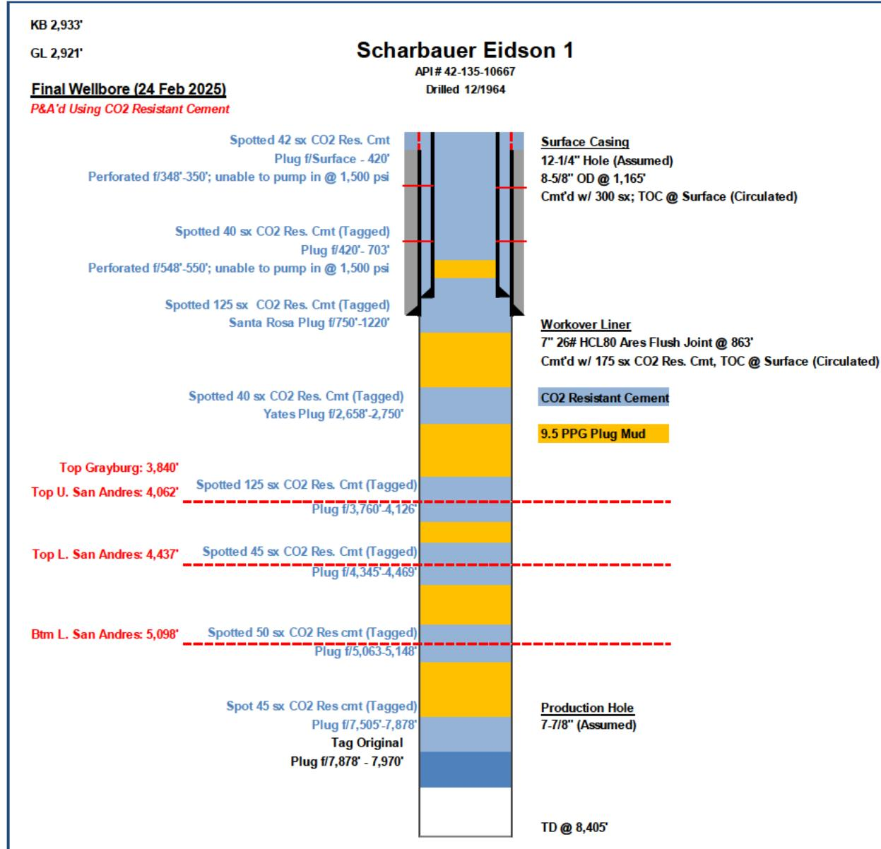
Figure 98. Wellbore diagram following corrective action on Scharbauer Eidson-1 (4213510667).
