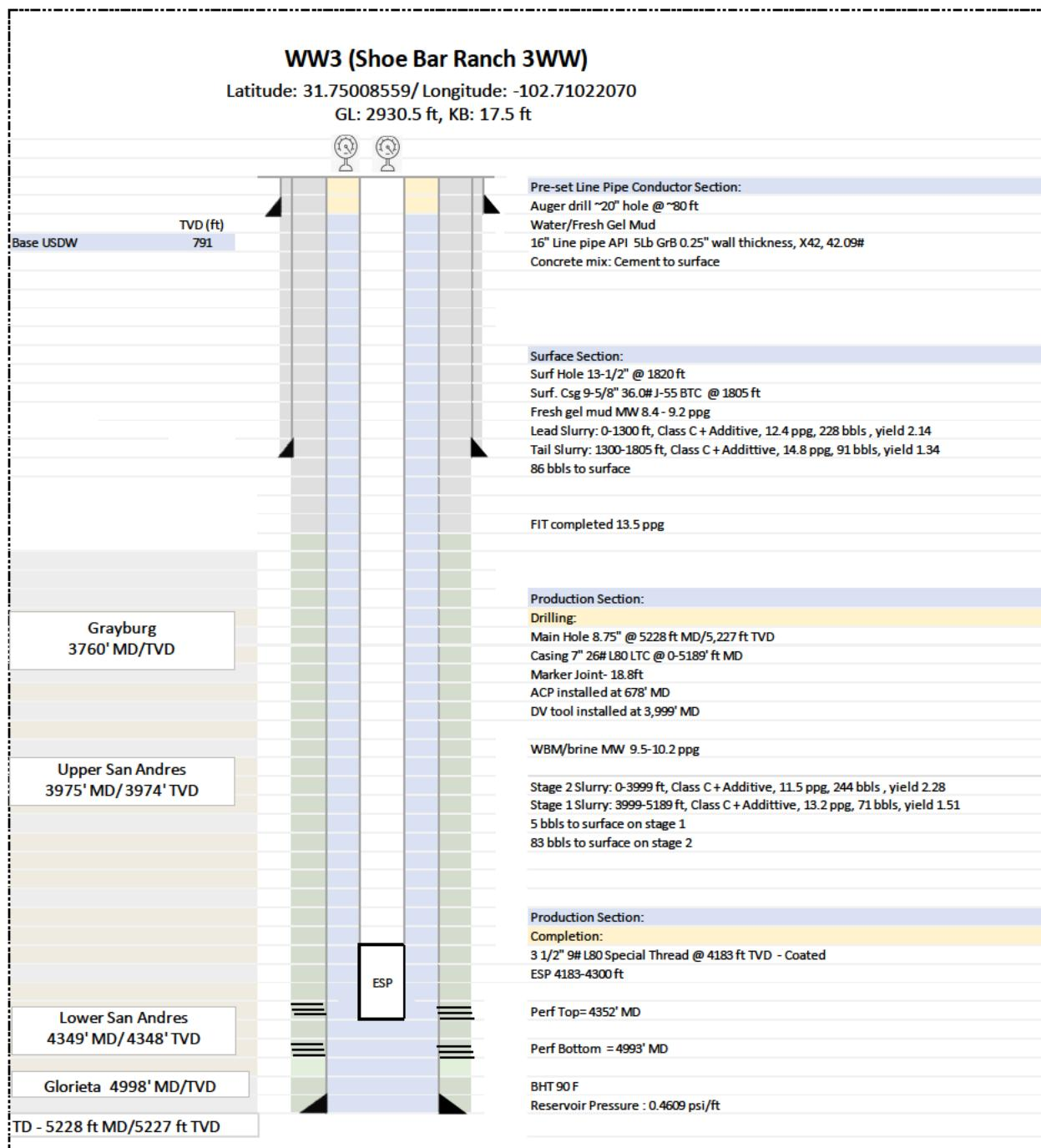
**Figure 8. As-built wellbore diagram for WW3.**
