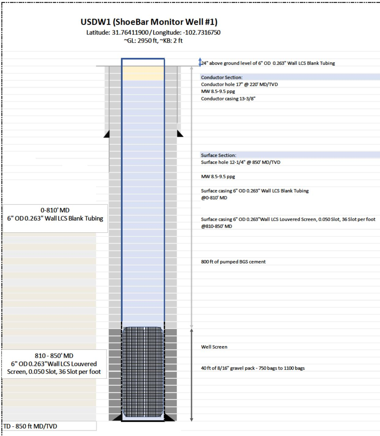
**Figure 5. As-built wellbore diagram for USDW1.**
