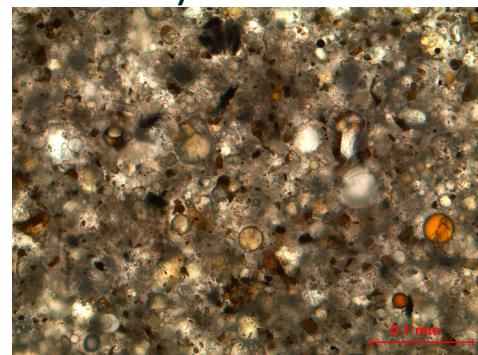
Fig. 1: Thin sections of set samples at 15.8 ppg (1893 kg/m<sup>3</sup>) under a light microscope.
