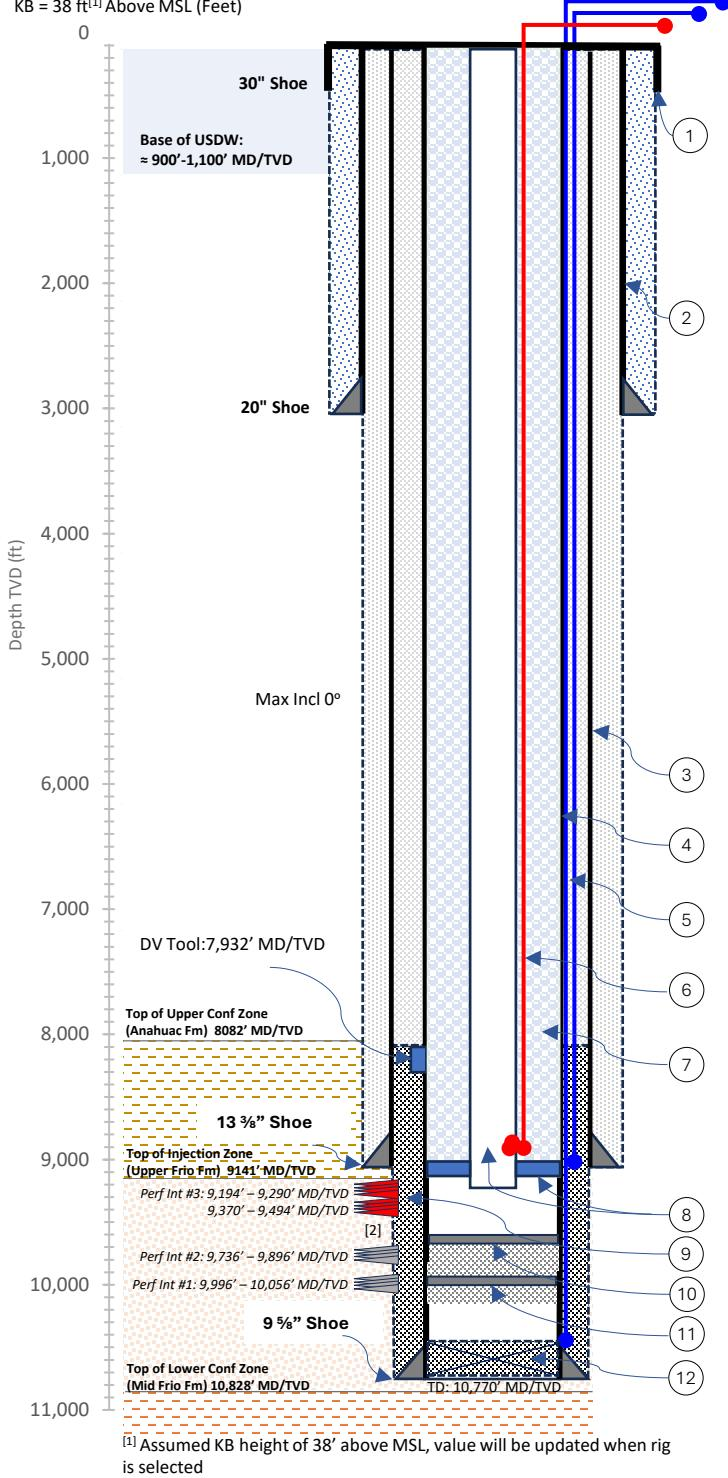
**1. 30" Conductor Pipe:** 1.0" WT, 28" ID, 310.3 lb/ft, X-56 Welded, plain-end, beveled conductor with drive shoe driven to refusal at 150' MD/TVD
