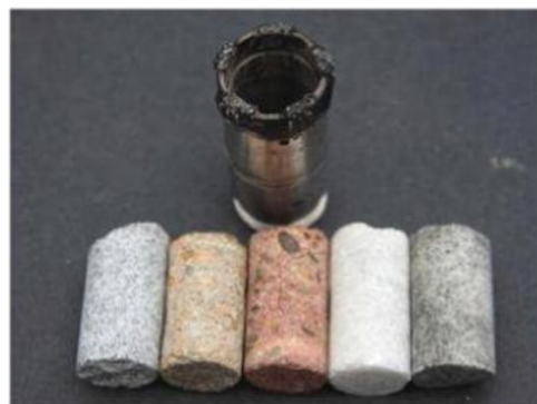
High-quality, uniformly sized core samples.
