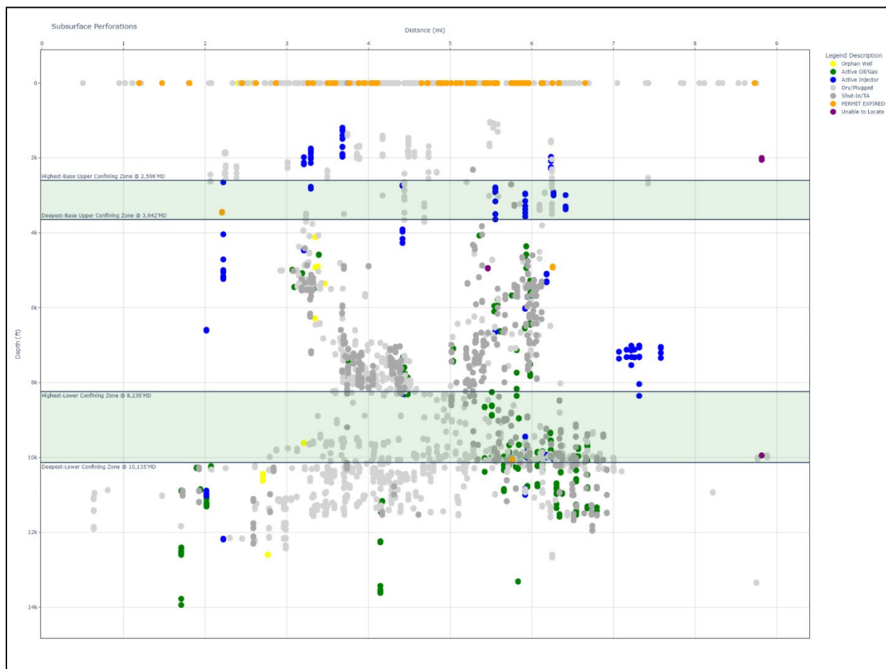
Figure 1-63 – Well perforation distribution in relation to the injection zone; the range of depths for the upper and lower confining zones in the project area are represented by the shaded green areas.
