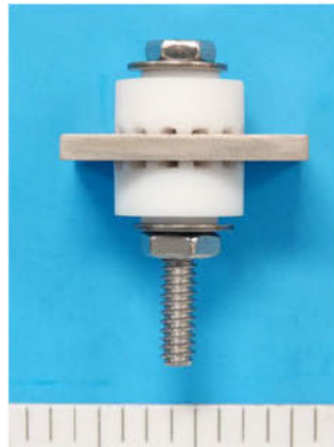
Figure CON-13: Crevice corrosion coupon assembly.
