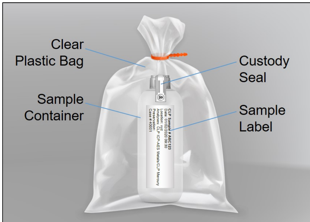
Figure 7-1. Packaged Sample with Identification and Chain of Custody Documentation (Excluding TR/COC Record)
