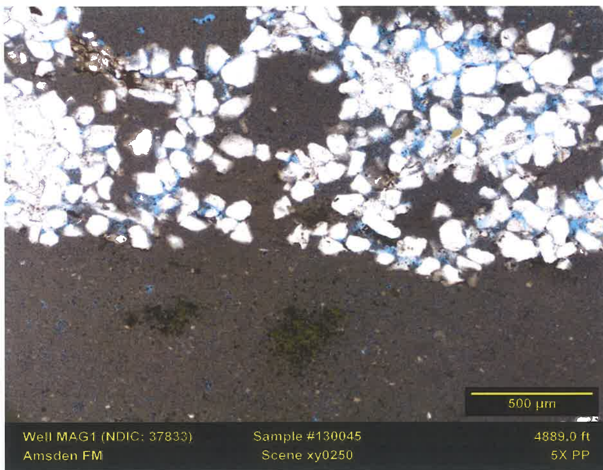
Figure 2-48. Thin section in the Amsden Formation. This interval shows a fine micritic dolomite with minor quartz grains. Porosity is generally low and found to be intergranular or due to the dissolution of dolomite in this example.
