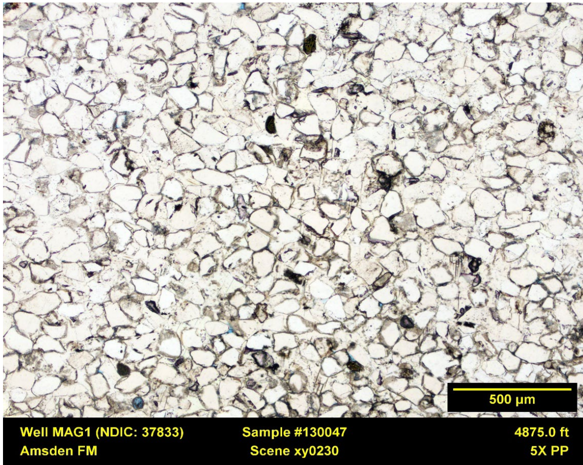
Figure 2-47. Thin section in the Amsden Formation. This interval is dominated by anhydrite and quartz. In this example, quartz grains are tightly cemented, and almost no porosity is observed.
