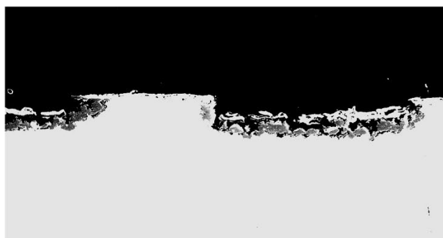
FIGURE 4. Shallow, film-covered local attack in carbon steel with 0.5 % chromium. 50 x.
