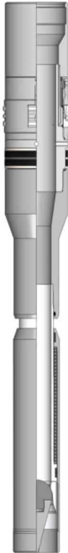
Figure 4-2: Safety Injection Valve
