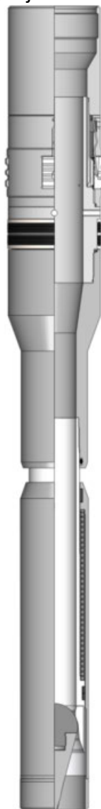
Figure 4-2: Safety Injection Valve
