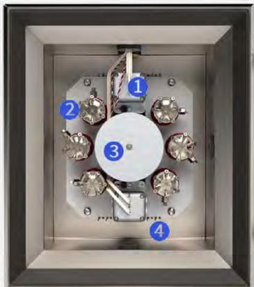
1. Thermal Conductivity Detector (Max 2)
