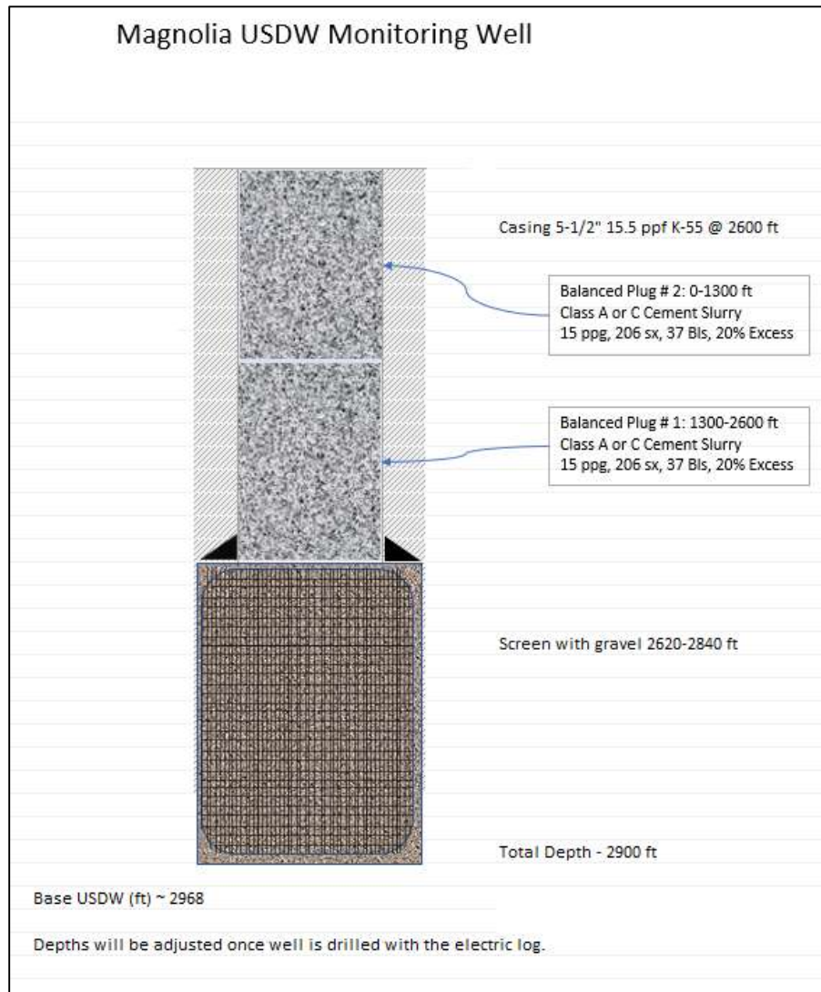
Figure PLG-12—Magnolia USDW 2 cement plug information.
