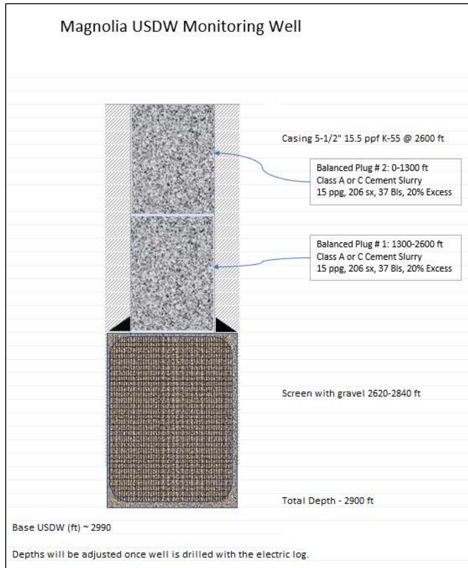
Figure PLG-11—Magnolia USDW 1 cement plug information.
