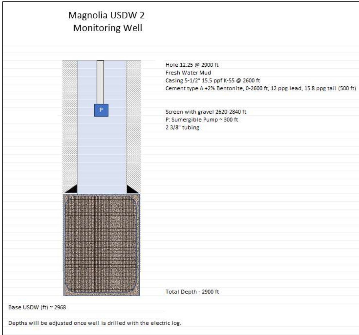
Figure CON-35—Proposed Magnolia USDW 2 wellbore diagram
