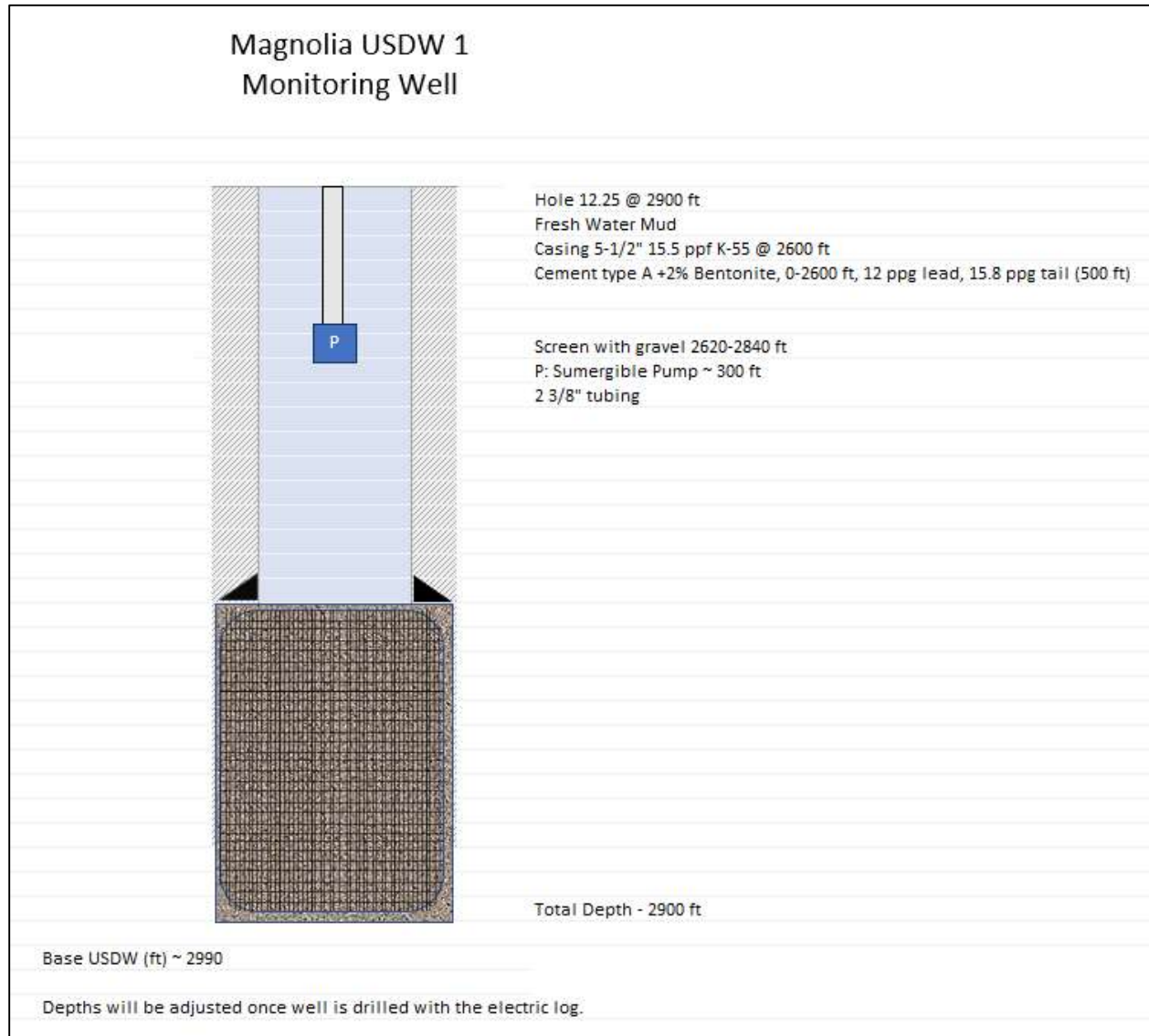
Figure CON-34—Proposed Magnolia USDW 1 wellbore diagram
