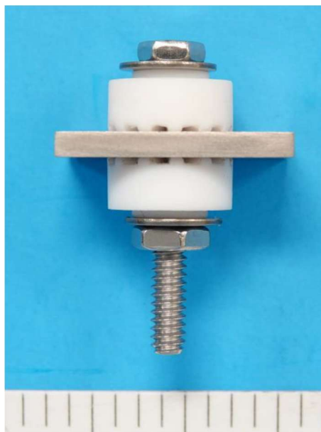
Figure CON-17—Crevice corrosion coupon assembly
