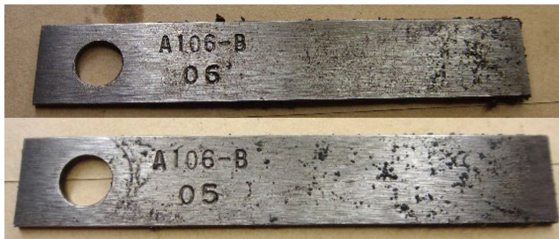
Figure 1: Corrosion Coupon A106-B Q3-2022 (top figure) and Q4-2022 (bottom figure) shows particulates adhering to coupons indicative of upstream corrosion.
