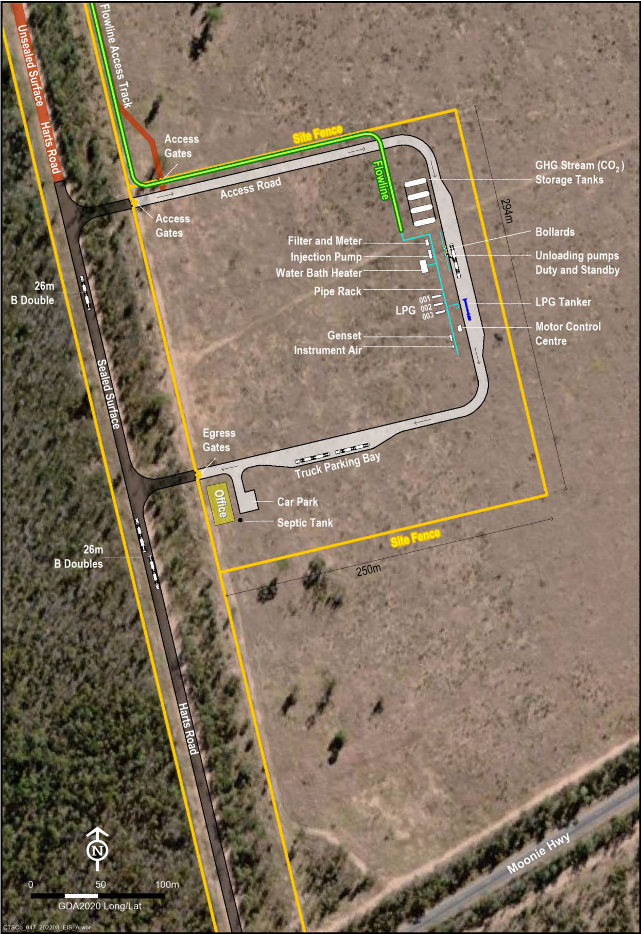
Figure 2-18 Transportation Facility (general arrangement plan)
