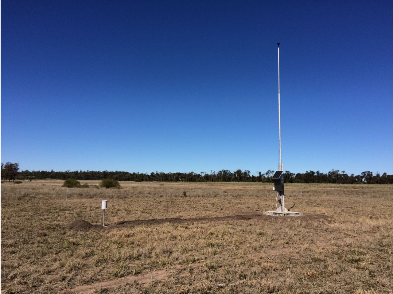
Figure 2-17 Indicative Air Quality and Atmospheric Monitoring Station (top of mast is 10 m above ground level)
