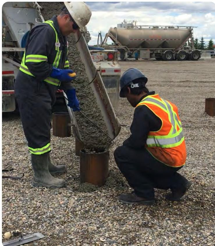
Carbon Upcycling partnered with **Burnco**, a North American leader in building materials, to deploy 140 m<sup>3</sup> of active concrete highway for the study. The innovative mixture was composed of 10% limestone and 30% reclaimed fly ash enhanced by Carbon Upcycling's carbon capture and utilization process, and was compared to an untreated control mix alongside 14 other mix designs.
