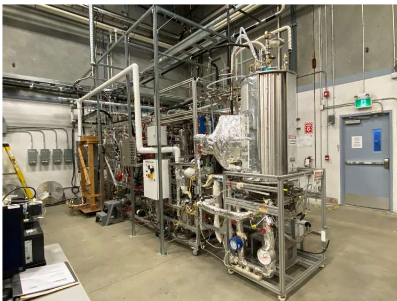
Figure 10: Process Demonstration Unit (PDU) at 0.1 TPD CO 2 capture capacity
