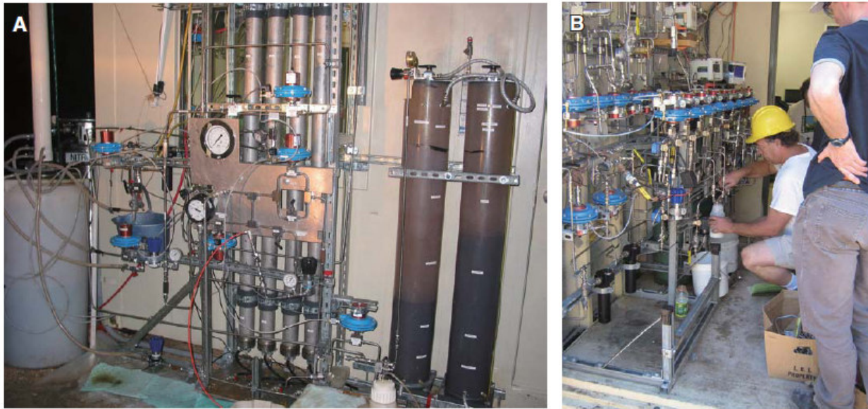
Figure 52. The Frio brine pilot surface sampling systems. (A) Four 13 L high pressure sample vessels mounted in sliding sleeves and resting on strain gauges to measure fluid density. (B) Computer-operated valve manifolds used to operate the U-tube samplers (see Footnote 18)
