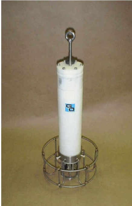
Figure 5. CDT probe for water column profiling acquisition 5
