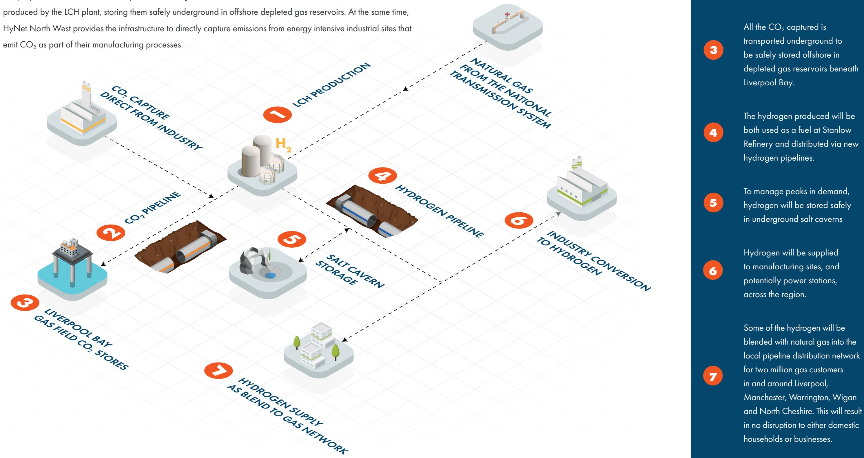
Natural gas will be fed into our LCH plant at Stanlow Refinery. The process splits this into hydrogen and CO<sub>2</sub>, around 95% of which is captured for safe storage.
