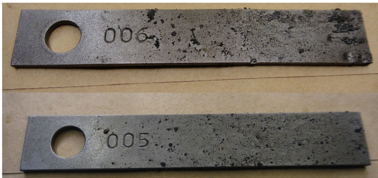
Figure 6: Corrosion Coupon 13CR-L80 Q1-2023 (top figure) and Q2-2023 (bottom figure) shows particulates adhering to coupons.
