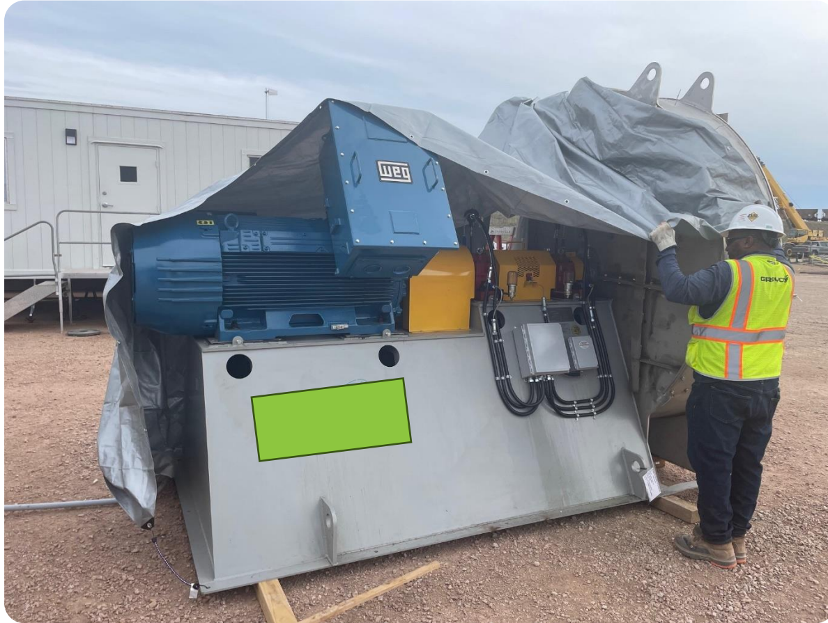
Process Equipment arrives – Flue gas blower
