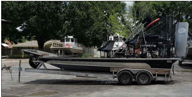
AIRBOAT DRILLING RIG 8'-0" X 22'-0" (DRAFT 2.0 FEET)
