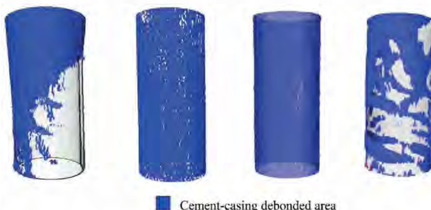
Figure 1: Examples of experimentally obtained, real microannuli geometries (Figure from Vrålstad and Skorpa, 2020)
