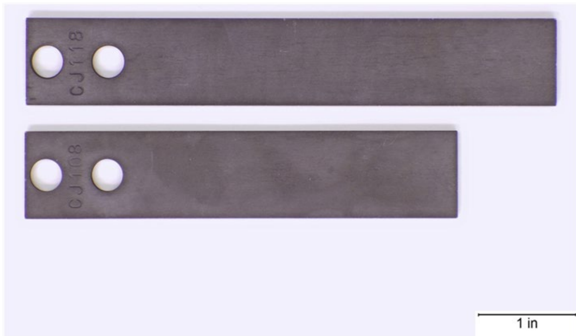
Figure 8: Type of corrosion coupons to be used for corrosion monitoring (Cosasco, 2022).
