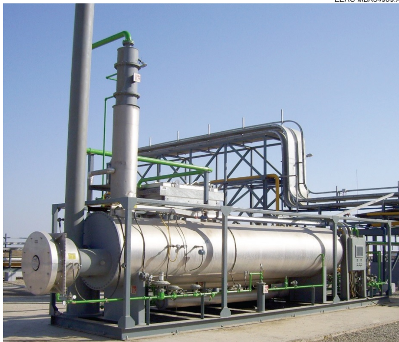
Figure 10. A TEG dehydration system (image from Q.B. Johnson Manufacturing, 2012).
