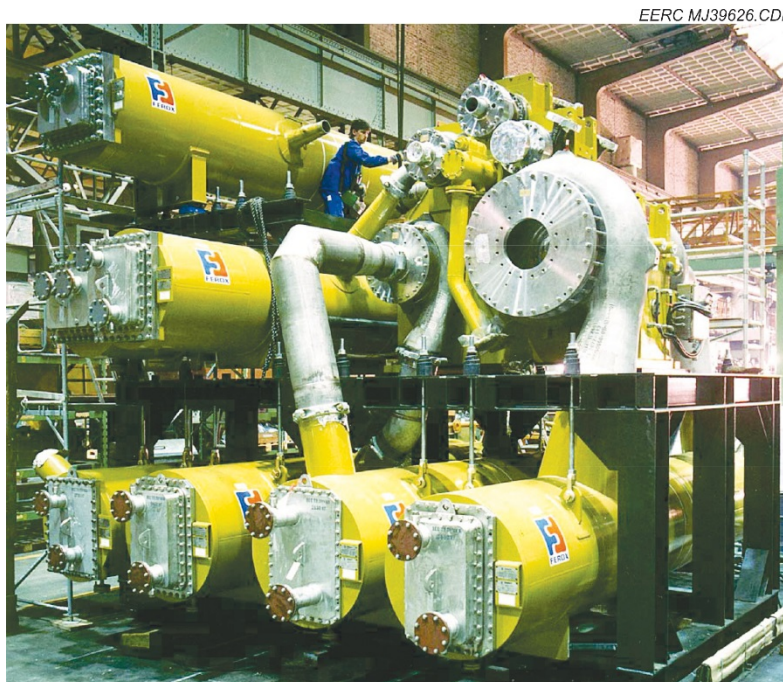
Figure 11. A ten-stage integrally geared centrifugal compressor with its intercoolers.
